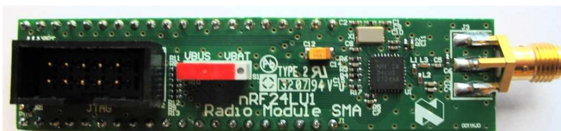
Figure 21 -The nRF24LU1 Radio Module with SMA connector
