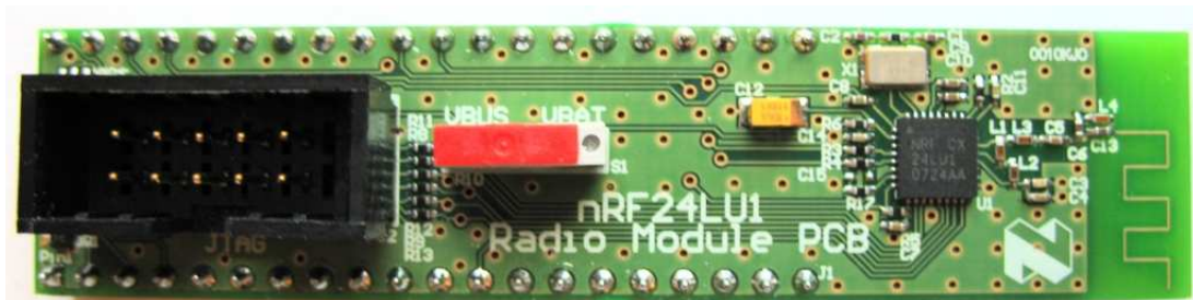
Figure 20 - The nRF24LU1 Radio Module with PCB antenna
