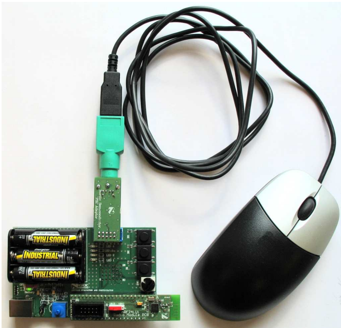
Figure 13: Basic Feature Board with PS/2 Adapter and nRF24LU1 Radio Module connected to a PS/2 Mouse
