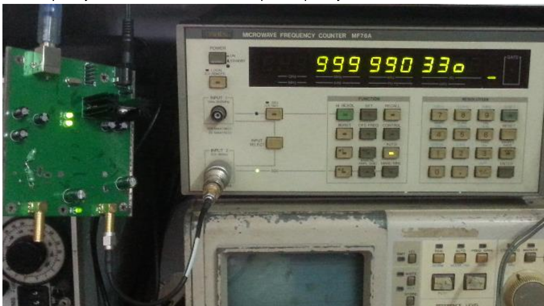
Test output frequency in this case 999.990 330MHz
