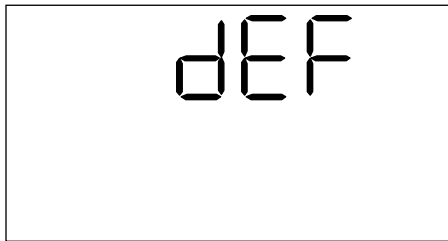
Figure 12. Restoring the Factory Defaults
