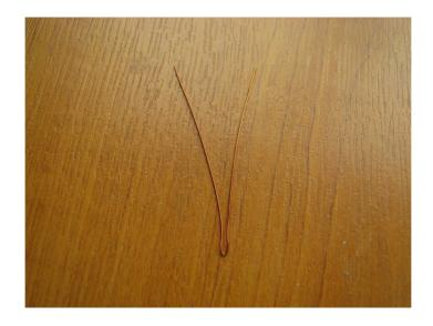
Twist some 8-10mm from the end together, to prevent slipping into the core:
