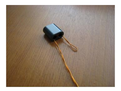
Complete the transformer by pushing a second turn, then cut-off the excess wire:
