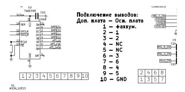
The location of contacts is shown as they are seen on the main board. Additional modules may be connected to power and other signals. For example, the C76 capacitor is located near the battery connector. The upper part of C76 is GND, the lower part is "+".
