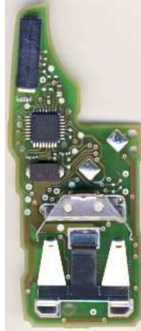
Picture 22: 5FA 010 185-11 and FS09A32 PCB back
