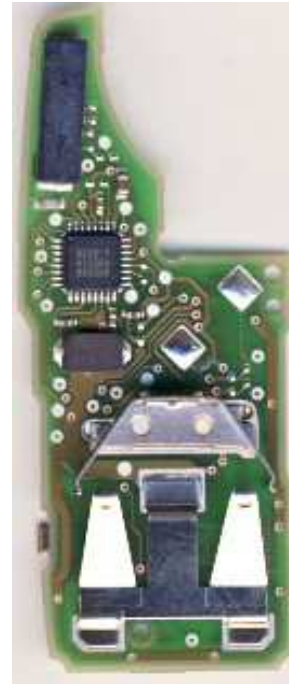
Picture 17: 5FA 010 185-06 and FS09A31 PCB back
