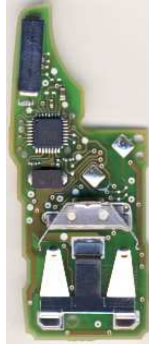
Picture 27: 5FA 010 185-16 and FS09A33 PCB back
