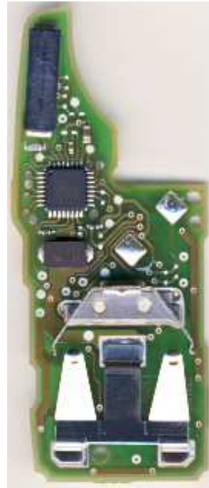
Picture 12: 5FA 010 185-01 and FS09A30 PCB back
