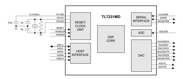
Figure 2. Functional Block Diagram of TL7231MD
