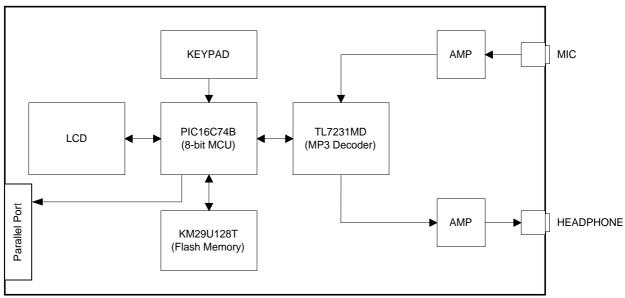
Figure 3. Block Diagram of TL7231MD Reference Board
