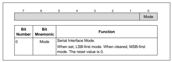
Figure 10. Serial Interface Mode reported through HDO5
