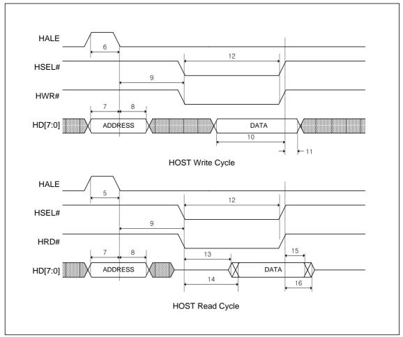
Figure 20. Timing for Host Interface Port pins
