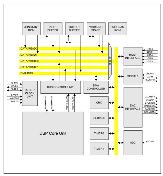
Figure 1. Functional Block Diagram of TL7230MD
