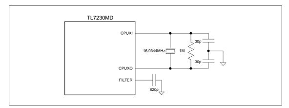
Figure 3. Clock Circuit
