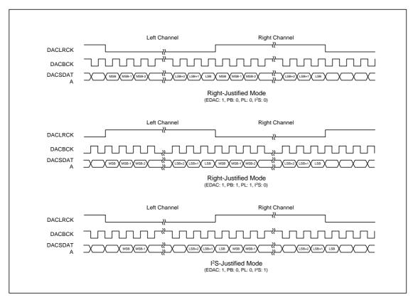
Figure 16. Examples of External DAC Interfaces
