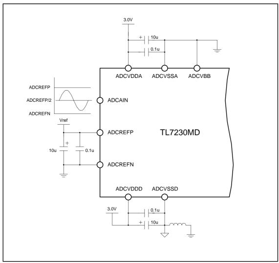
Figure 17. Reference Circuit when using internal ADC
