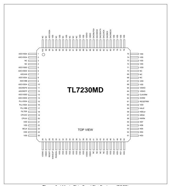
Figure 2. 100-pin Thin Quad Flat Package (TQFP)
