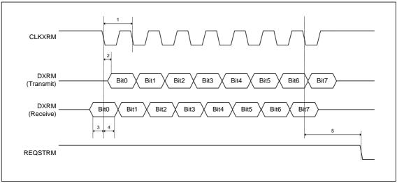
Figure 19. Timing for Serial Port in case of LSB-First Mode
