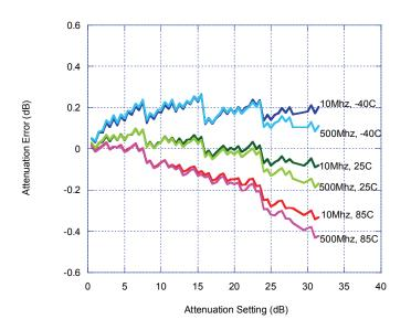
Figure 8. Attenuation Error Vs. Attenuation Setting
