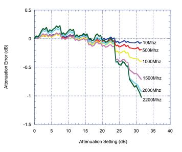
Figure 10. Attenuation Error Vs. Attenuation Setting
