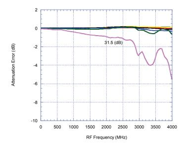
Figure 9. Attenuation Error Vs. Attenuation Setting
