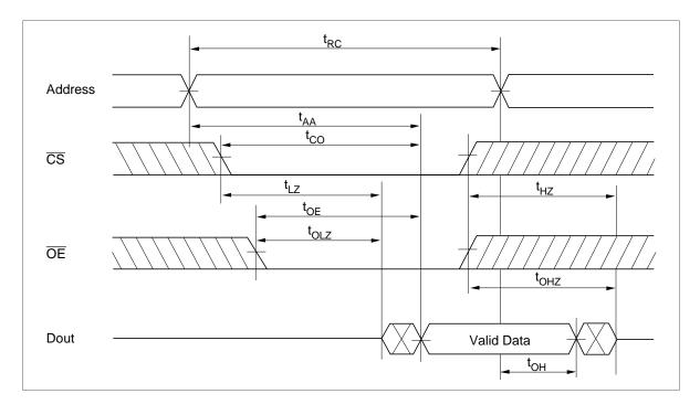
Read Timing Waveform  $(\overline{WE} = V_{IH})$
