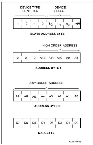
of the device select input pins. If the compare is not successful, no acknowledge is output during the ninth clock cycle and the device returns to the standby mode.
