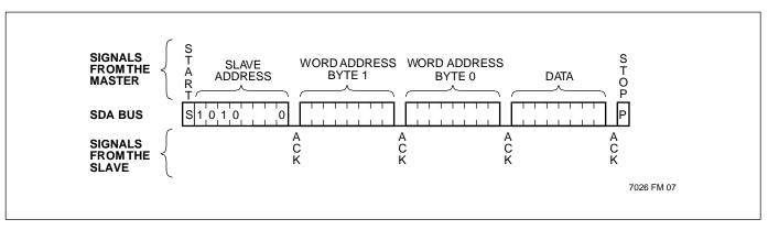
Figure 4. Byte Write Sequence
