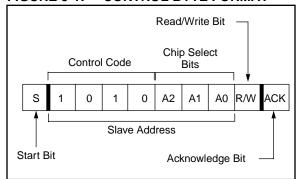
FIGURE 5-2: ADDRESS SEQUENCE BIT ASSIGNMENTS
