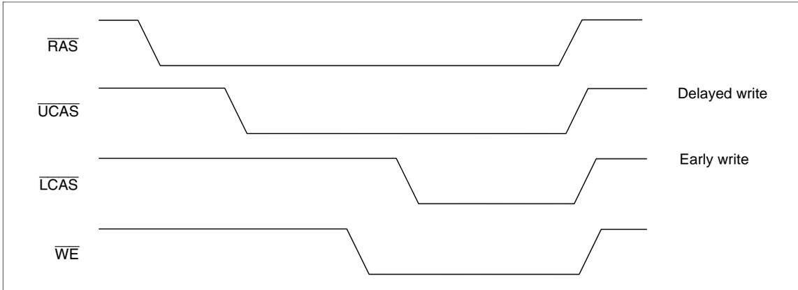
3. Closely separated upper/lower byte control is not allowed. However when the condition ( $t_{\text{CP}} \leq t_{\text{UL}}$ ) is satisfied, EDO page mode can be performed.
