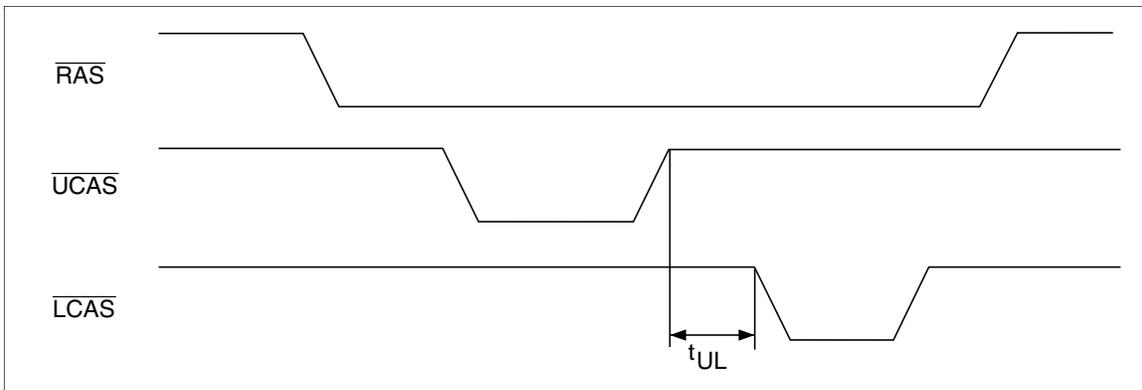
4. Byte control operation by remaining  $\overline{\text{UCAS}}$  or  $\overline{\text{LCAS}}$  high is guaranteed.
