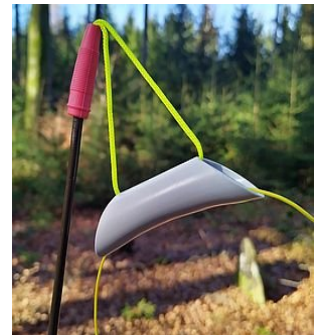
Figure 5: Top radiator wire support
