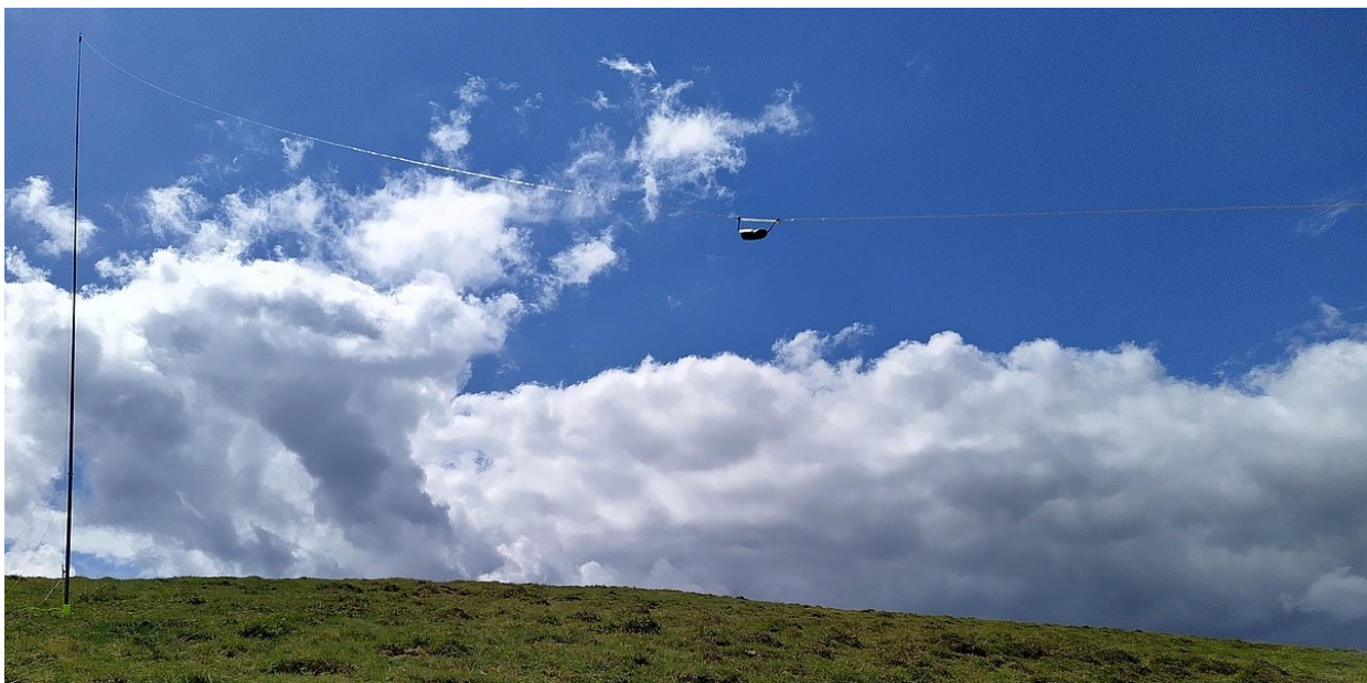
Figure 1: A typical inverted-L EFHW antenna setup with one bypassable loading coil
