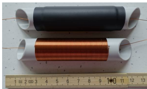
Figure 35: Building the 80-meter-band loading coil
