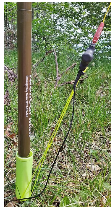
Figure 46: Holding the coupler in place with a cord
