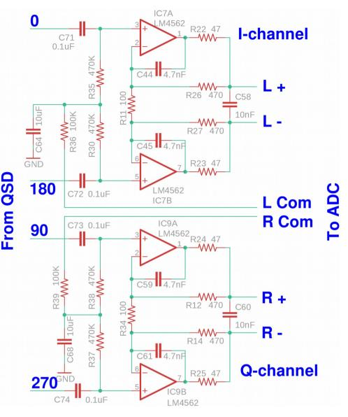
performance than the AK5386 but the PCM1804 has a differential input. One input could be ignored, feeding the I and Q signals into only one terminal of each ADC (left and right); however, this would sacrifice 6dB of the potential 112dB claimed dynamic range of the PCM1804.
