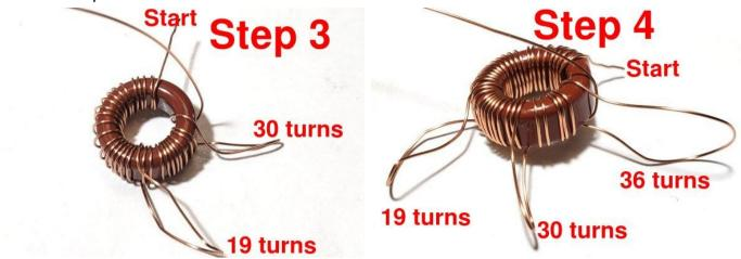
Step 5: Wind the remaining turns to complete the total of 41 turns.
