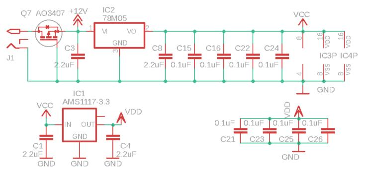
The two fixed voltage regulators in the QDX design produce +3.3V and +5.0V. The +5V voltage regulator type is 78M05 and the 3.3V type is AMS1117.
