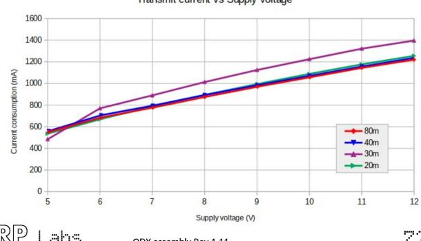
Transmit current vs Supply voltage
