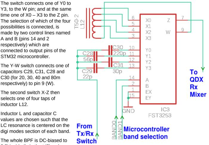
2.5V midrail via the trifilar phase splitting transformer T2 of the Receive mixer.
