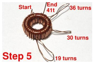
**<u>Step 6</u>**: Now with a pair of pliers, you can squeeze each of the loops into a sharp point, such that it is easy to fit through the large holes at the 19, 30 and 36-turn taps (see photo, right).
