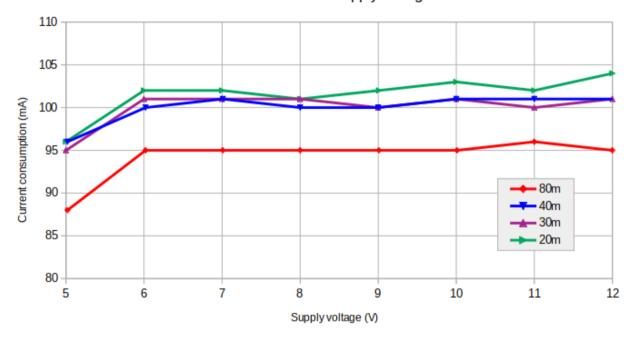
Receive current vs Supply voltage
