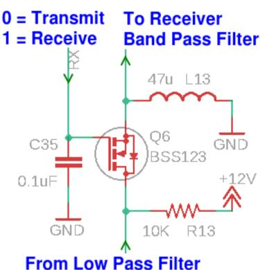
switches the MOSFET on or off. Capacitor C35 close to the MOSFET gate is found to be necessary to prevent inductive pickup of the 5W RF from partially switching on the MOSFET.
