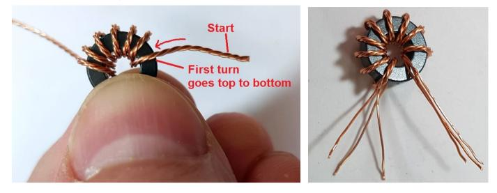
Now it's necessary to identify which wire belongs to which winding. You have three windings twisted together, they all use the same wire. The only way to do this is with a DMM as continuity tester. First, untwist and straighten the wire ends that are not wound around the toroidal core.
