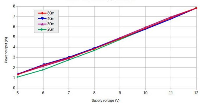
Power output vs Supply voltage
