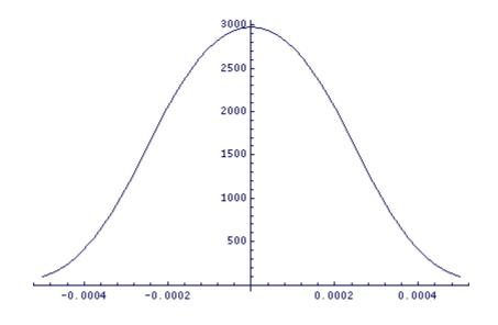
The truncated and scaled impulse response of the Gaussian low-pass filter.
