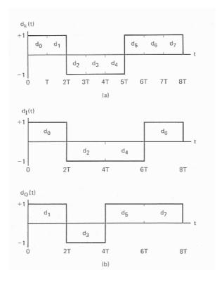
A convenient orthogonal realisation of a QPSK waveform , s(t) is achieved by amplitude modulating the in-phase and quadrature data streams onto the cosine and sine functions of a carrier wave as follows:
