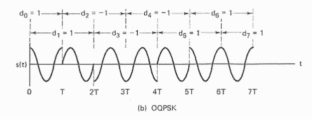
When an OQPSK signal undergoes bandlimiting, the resulting intersymbol interference causes the envelop to droop slightly to the region of  $\pm 90^{\circ}$  phase transition, but since the phase transitions of 180 have been avoided in OQPSK, the envelop will never go to zero as it does in QPSK.
