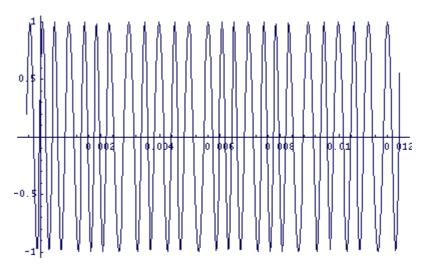
The GMSK modulated signal m(t) as in the second figure.
