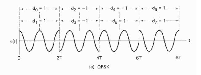
If a QPSK modulated signal undergoes filtering to reduce the spectral side lobes, the resulting waveform will no longer have a constant envelop and in fact, the occasional 180° shifts in phase will cause the envelope to go to zero momentarily.
