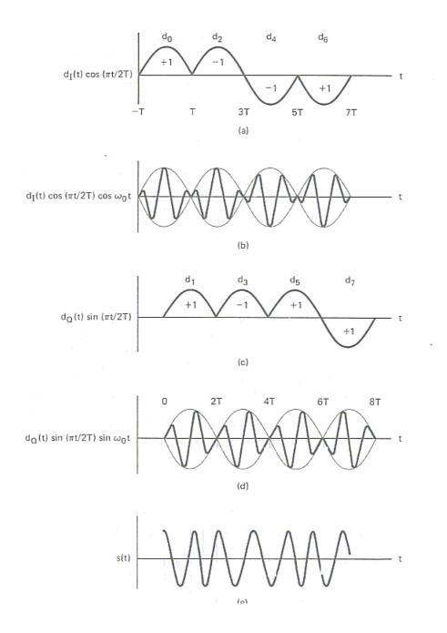
The MSK modulation makes the phase change linear and limited to  $\pm (\pi/2)$  over a bit interval T. This enables MSK to provide a significant improvement over QPSK. Because of the effect of the linear phase change, the power spectral density has low side lobes that help to control adjacent-channel interference. However the main lobe becomes wider than the quadrature shift keying.
