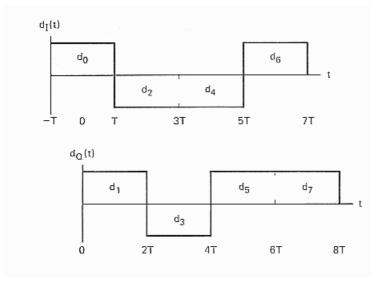
Thus the range of phase transitions is  $0^{\circ}$  and  $90^{\circ}$  (the possibility of a phase shift of  $180^{\circ}$  is eliminated) and occurs twice as often, but with half the intensity of the QPSK. While amplitude fluctuations still occur in the transmitter and receiver they have smaller magnitude. The bit error rate for QPSK and OQPSK are the same as for BPSK.
