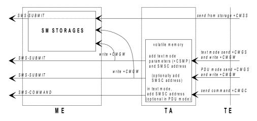
Figure 8: Message service send and write procedures
