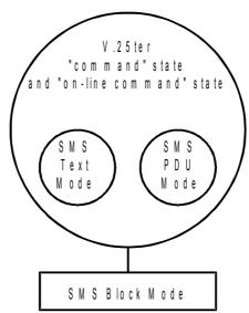
Figure 0.1/GSM 07.05: Block, Text and PDU modes
