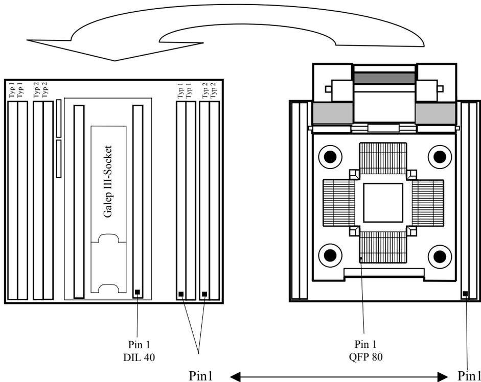
Please carefully note the correct orientation, when inserting the upper board into the lower board (see diagram above).
