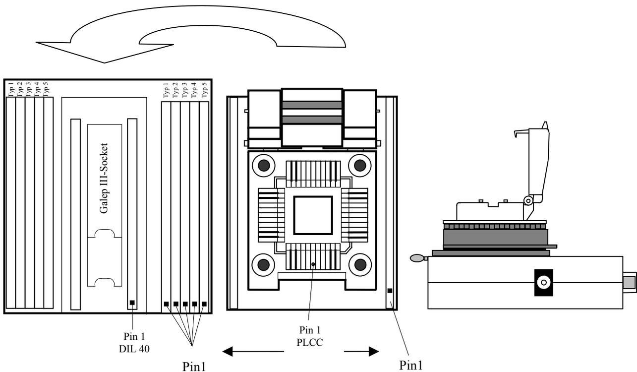
Please carefully note the correct orientation, when inserting the upper board into the lower board (see diagram above). The diagram also illustrates how the adapter will fit into the GALEP.
