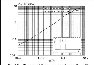
Fig. 10. Transient thermal impedance  $Z_{th} = f(t_p)$
