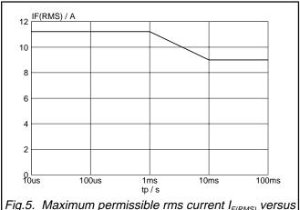
Fig.5. Maximum permissible rms current  $I_{F(RMS)}$  versus pulse width.
