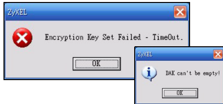
Figure 30 Incorrect DAK or No DAK
