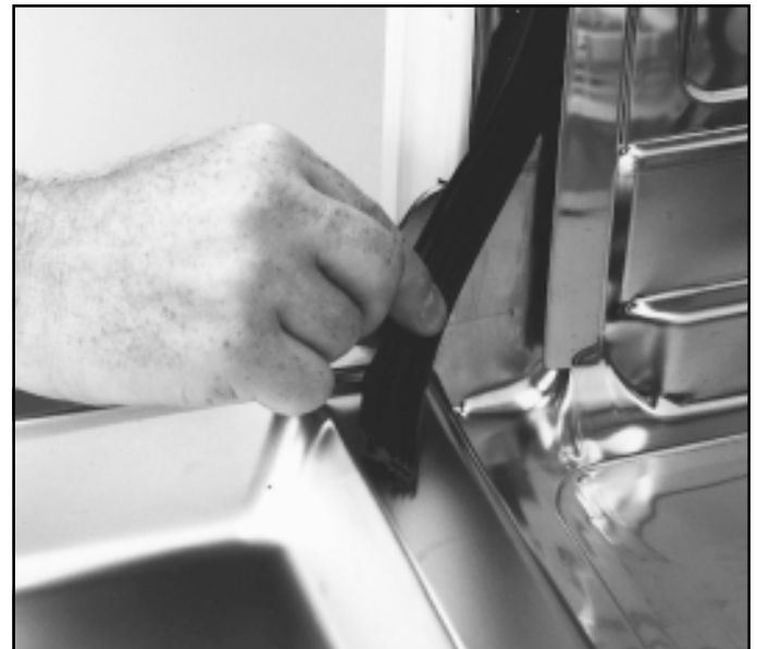
Fig. 5-6 To remove the Gasket, simply pull it away from the Tank Channel.
