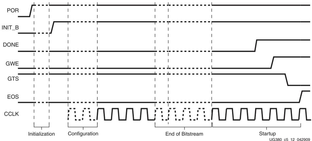
Figure 5-12: Configuration Signal Sequencing (Default Startup Settings)
