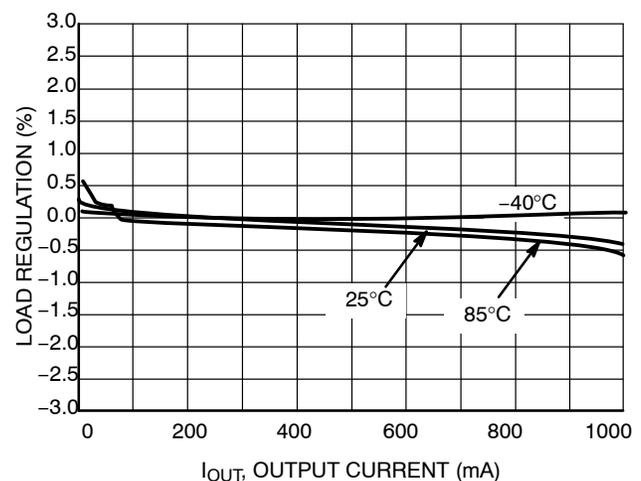
**Figure 29. Load Regulation vs. Output Current**
