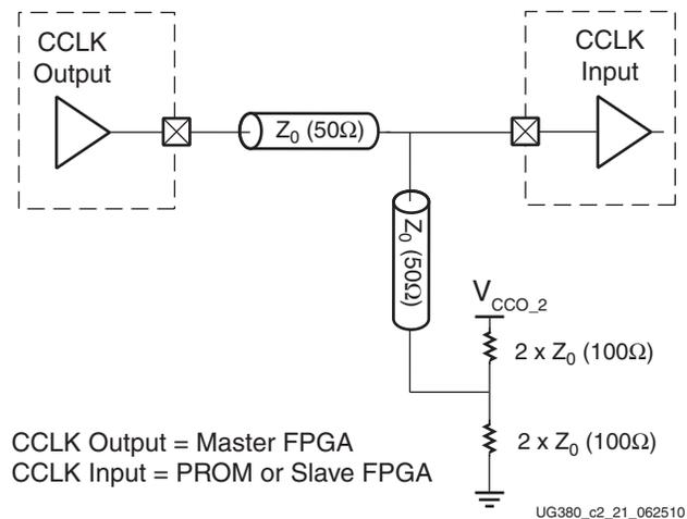
Figure 2-22: Point-to-Point: One CCLK Output, One CCLK Input
