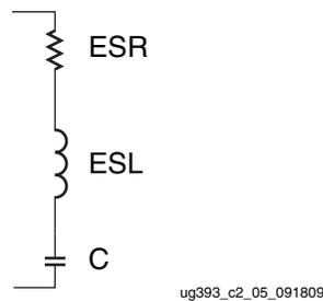
*Figure 2-5: Parasitics of a Real, Non-Ideal Capacitor*
