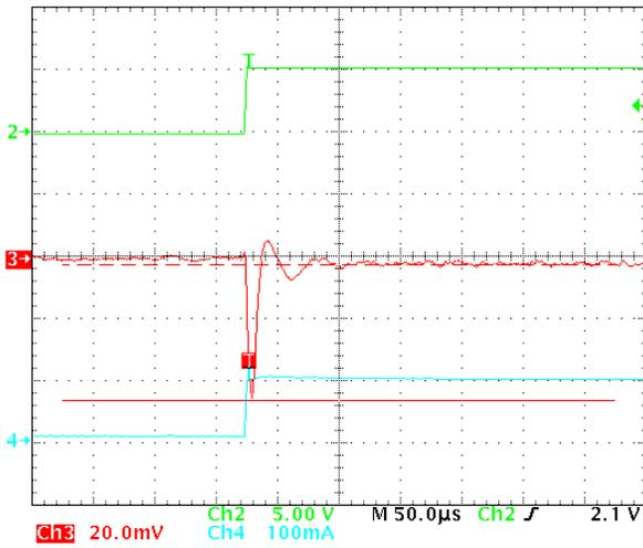
**Figure 17. 10 mA to 100 mA Load Transient in 1  $\mu\text{s}$**
