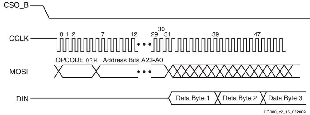
Figure 2-15: Master SPI Timing Diagram (opcode = 03h)
