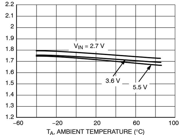
**Figure 14. Switching Frequency vs. Ambient Temperature**
