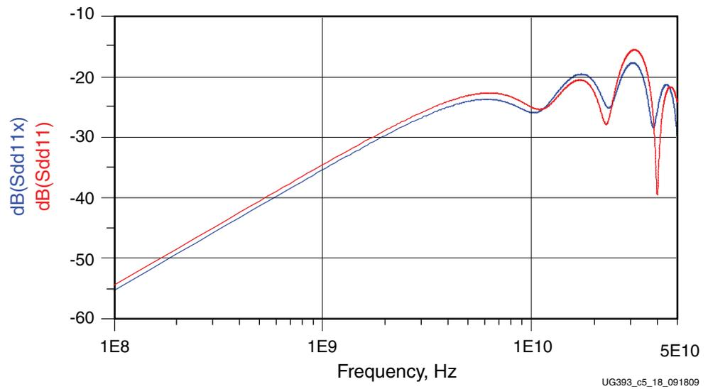
Figure 5-18: Simulated TDR of 45 Degree Bends with Jog-Outs
