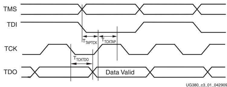
**Figure 3-1: Spartan-6 FPGA Boundary-Scan Port Timing Waveforms**
