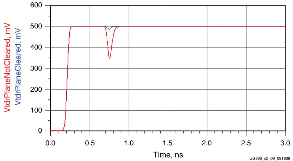
Figure 5-9: TDR Results Comparing 0402 Pad Structures
