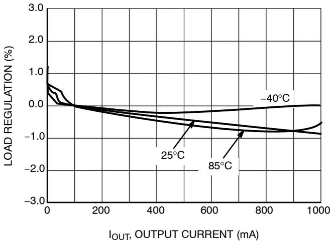
**Figure 15. Load Regulation vs. Output Current**
