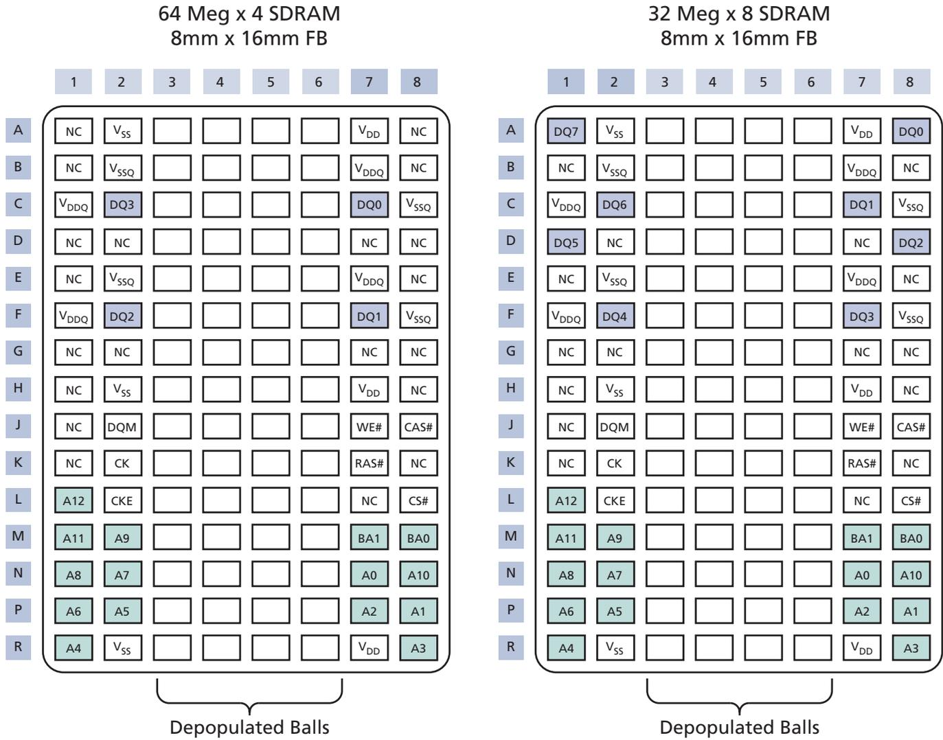
**Figure 6: 54-Ball VFBGA (Top View)**
