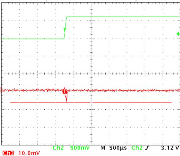
**Figure 19. 3.0 V to 3.6 V Line Transient, Rise = 50  $\mu\text{s}$**
