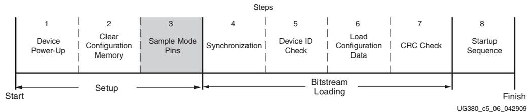
Figure 5-6: Sample Mode Pins (Step 3)
