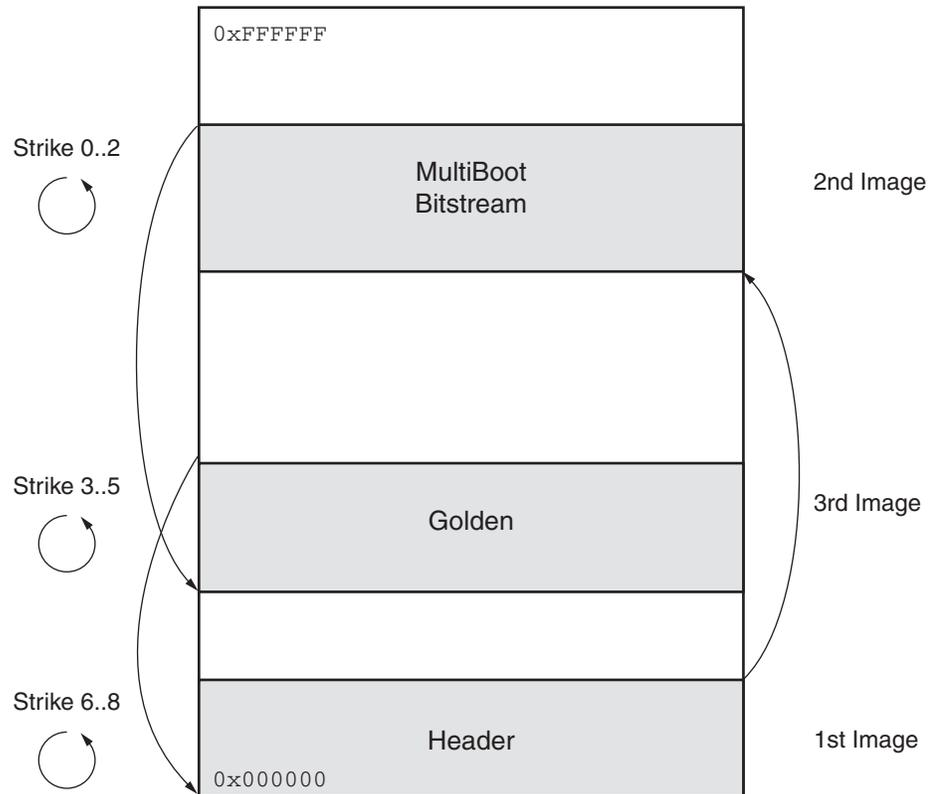
Figure 7-1: MultiBoot Logic
