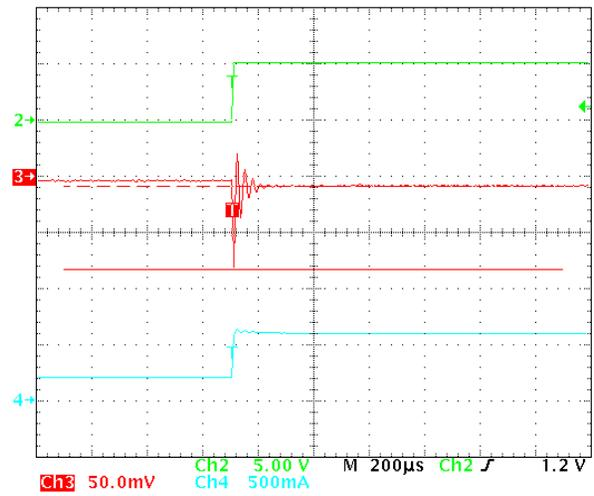
**Figure 18. 200 mA to 600 mA Load Transient in 1  $\mu\text{s}$**
