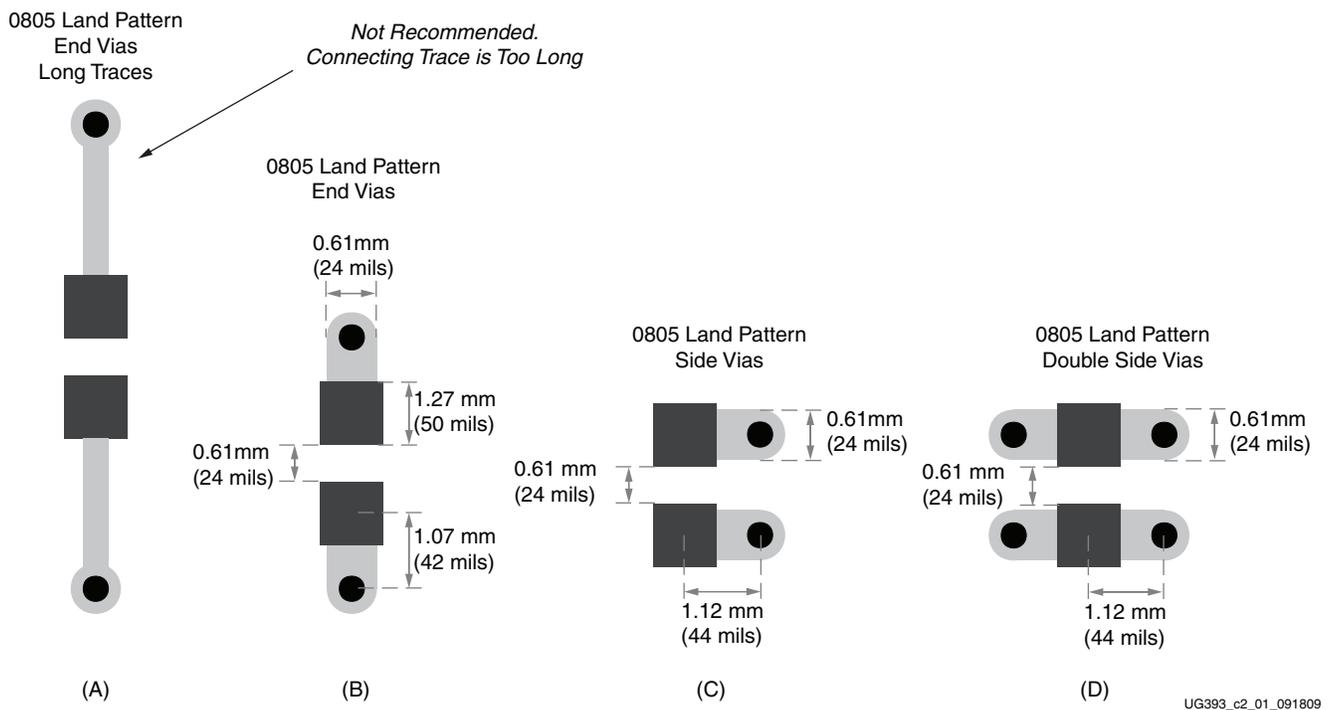
Figure 2-1: Example 0805 Capacitor Land and Mounting Geometries
