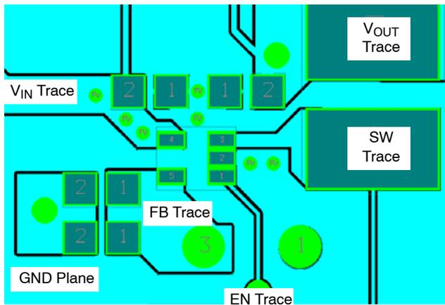
Figure 30. TSOP-5 Recommended Board Layout
