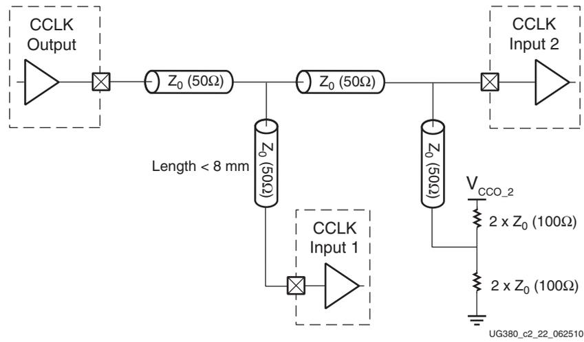
Figure 2-23: Multi-Drop: One CCLK Output, Two CCLK Inputs
