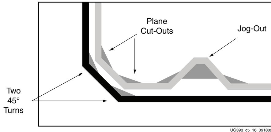
**Figure 5-16: Example Design for 90 Degree Bends in Traces**
