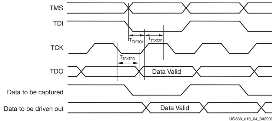
**Figure 10-4: Spartan-6 FPGA Boundary-Scan Port Timing Waveforms**
