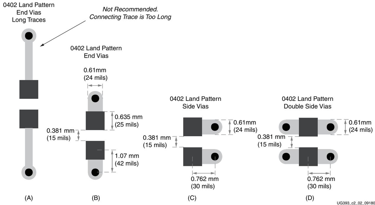
Figure 2-2: Example 0402 Capacitor Land and Mounting Geometries
