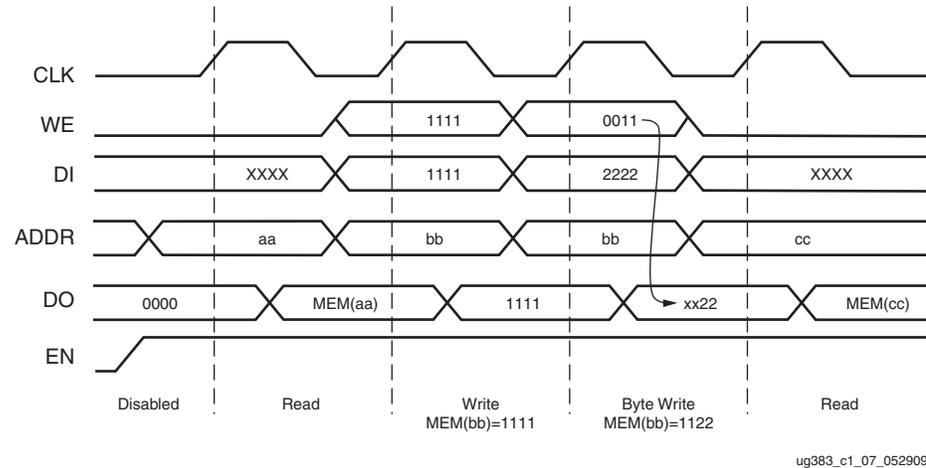
Figure 7: Byte-wide Write Operation Waveforms (x36 WRITE\_FIRST)
