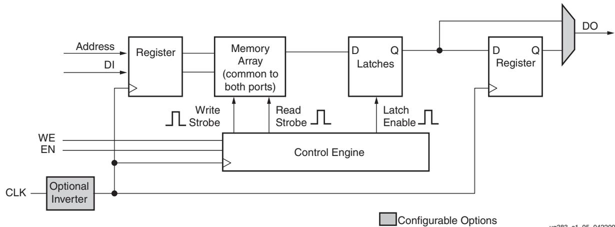
Figure 5: Block RAM Logic Diagram (One Port Shown)
