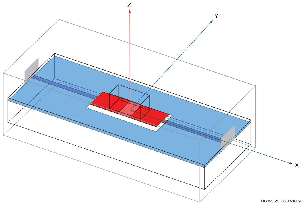
Figure 5-6: Ansoft HFSS Model of Pad Clear-Out
