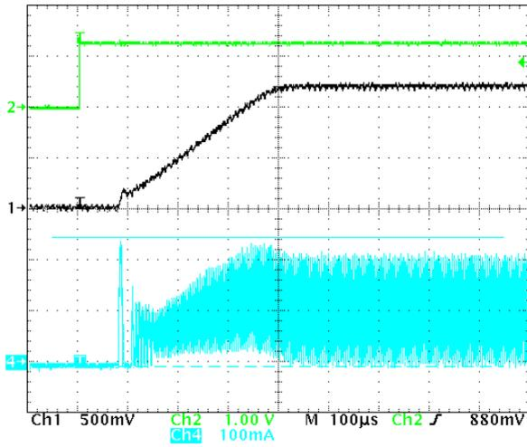
**Figure 21. Typical Soft-Start ( $V_{IN} = 3.6\text{ V}$ ,  $V_{OUT} = 1.2\text{ V}$ ,  $I_{OUT} = 100\text{ mA}$ , Temperature =  $25^\circ\text{C}$ )**
