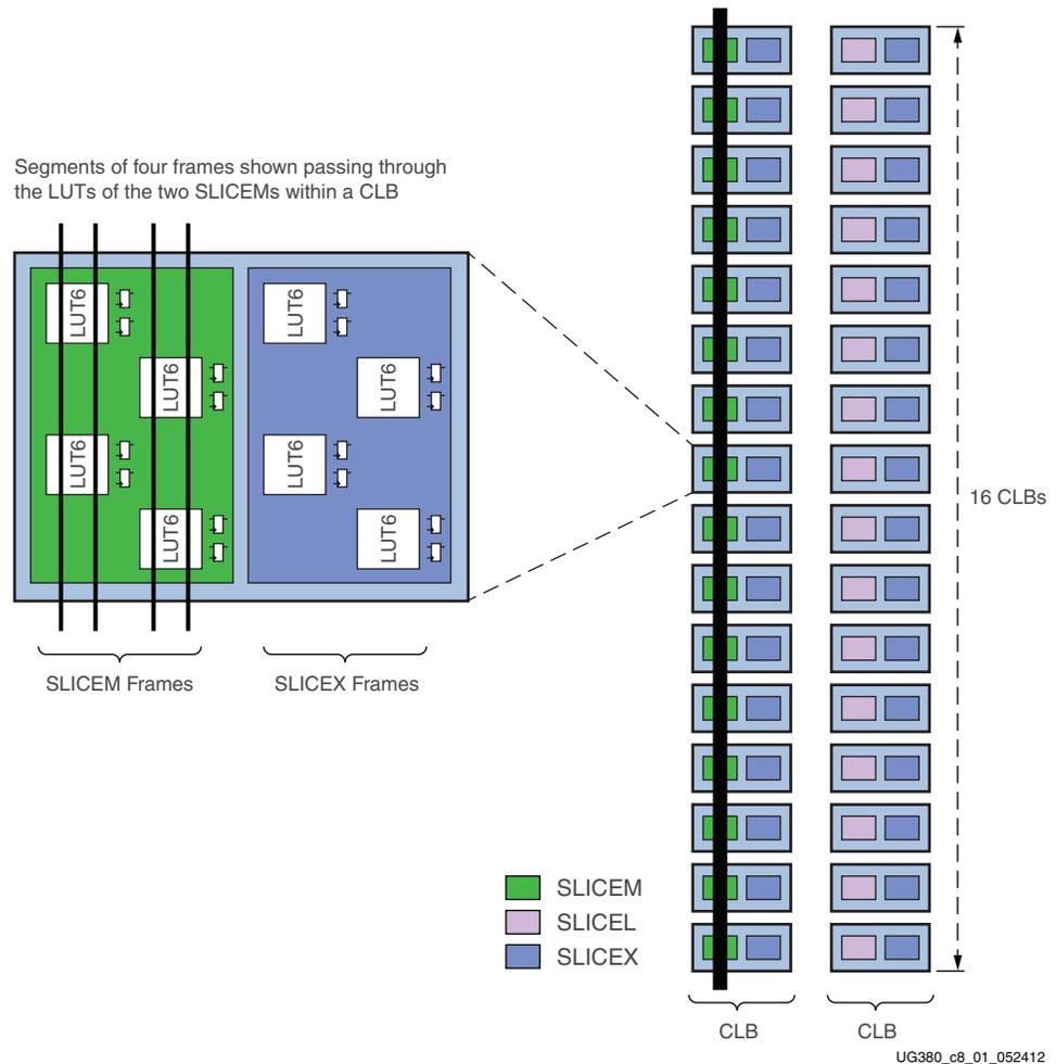
**Figure 8-1: CLB Frame Masking with Distributed RAM**
