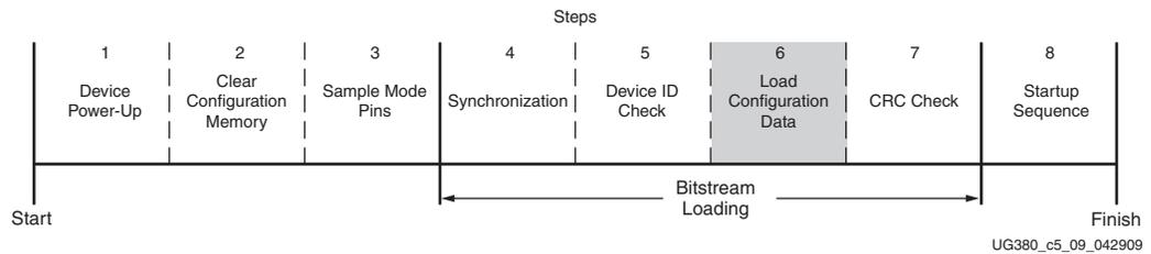
Figure 5-9: Load Configuration Data Frames (Step 6)
