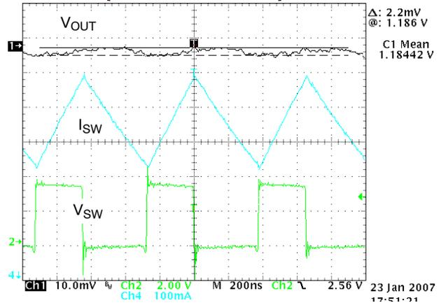
Figure 26. PWM Switching Waveforms
