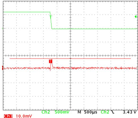
**Figure 20. 3.6 V to 3.0 V Line Transient, Fall = 50  $\mu\text{s}$**
