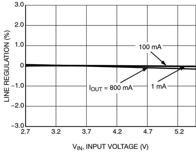
**Figure 16. Line Regulation vs. Input Voltage**
