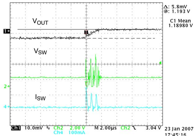
Figure 27. PFM Switching Waveforms
