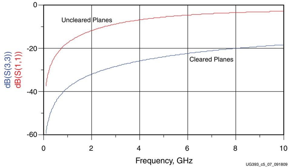
Figure 5-7: Return Loss Comparison Between 0402 Pad Structures
