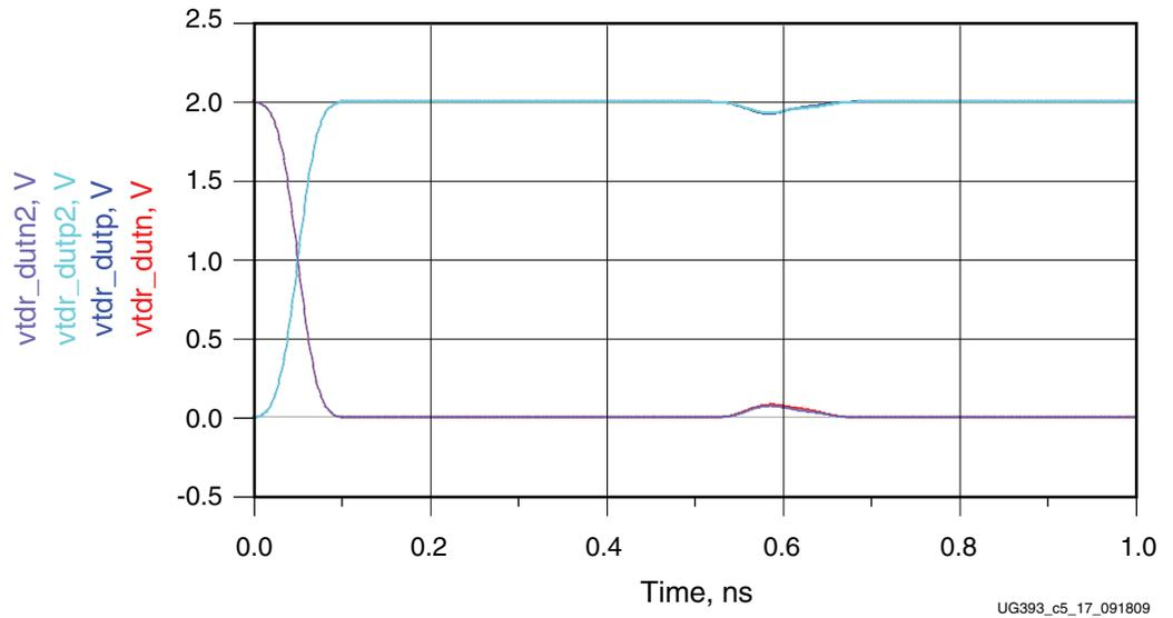
Figure 5-17: Simulated TDR of 45 Degree Bends with Jog-Outs
