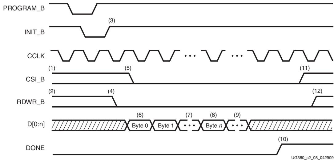
**Figure 2-8: Continuous x8 or x16 SelectMAP Data Loading**
