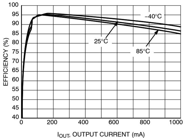
**Figure 28. Efficiency vs. Output Current**
