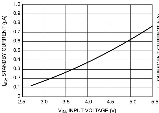
**Figure 9. Standby Current vs. Input Voltage**
