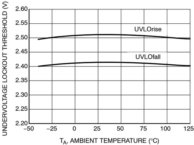
**Figure 23. Undervoltage Lockout Threshold vs. Ambient Temperature**
