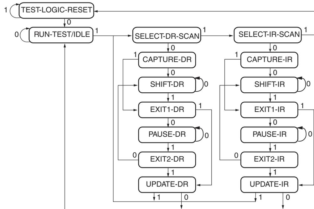
Note: The value shown adjacent to each state transition represents the signal present at TMS at the time of a rising edge at TCK.
