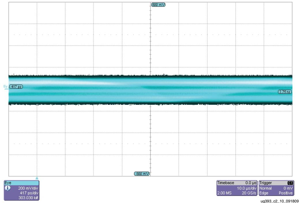
Figure 2-10: Infinite Persistence Measurement of Same Supply
