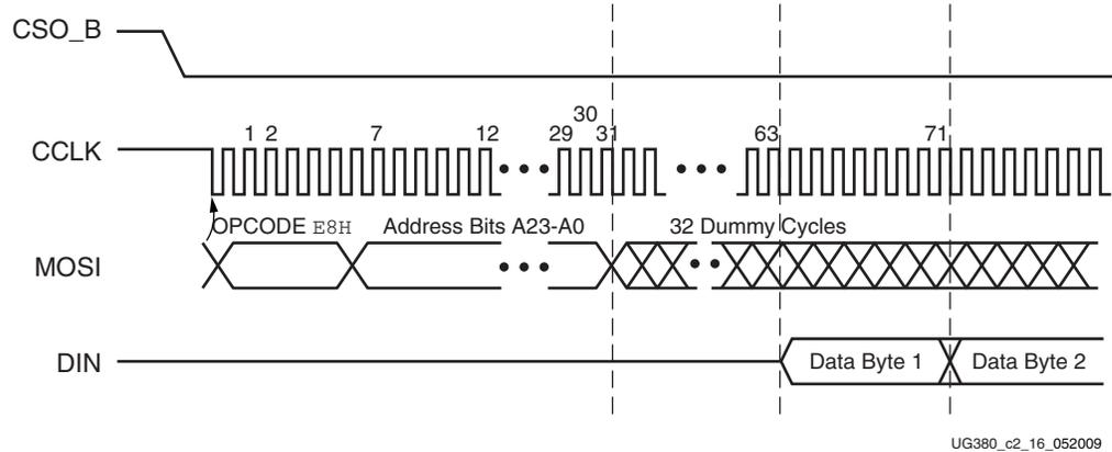
Figure 2-16: Master Serial SPI Timing Diagram (opcode = E8h)
