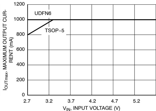
Figure 7. Maximum Output Current,  $T_A = 45^{\circ}C$
