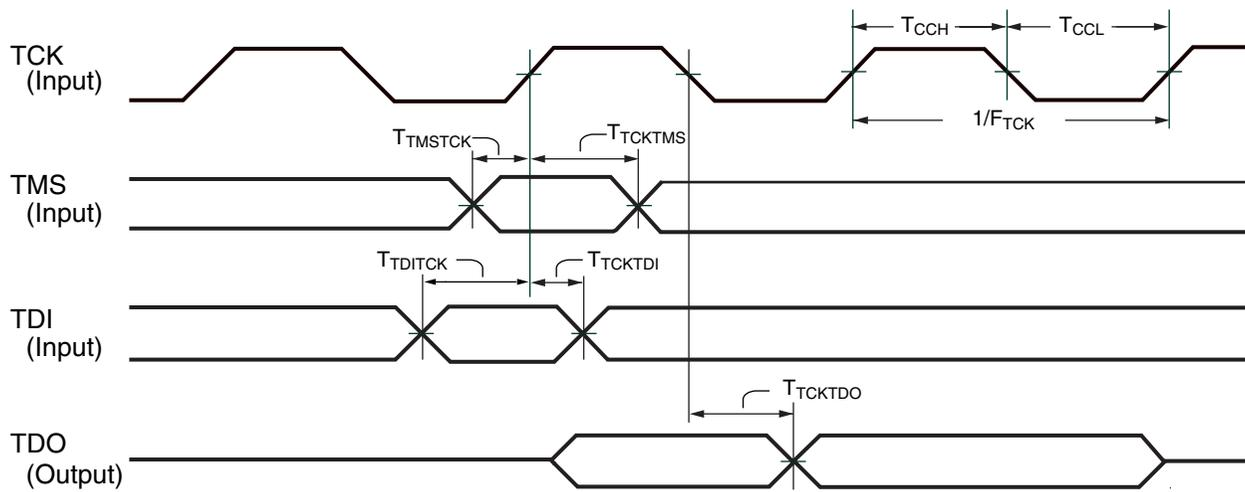
Figure 8: JTAG Waveforms
