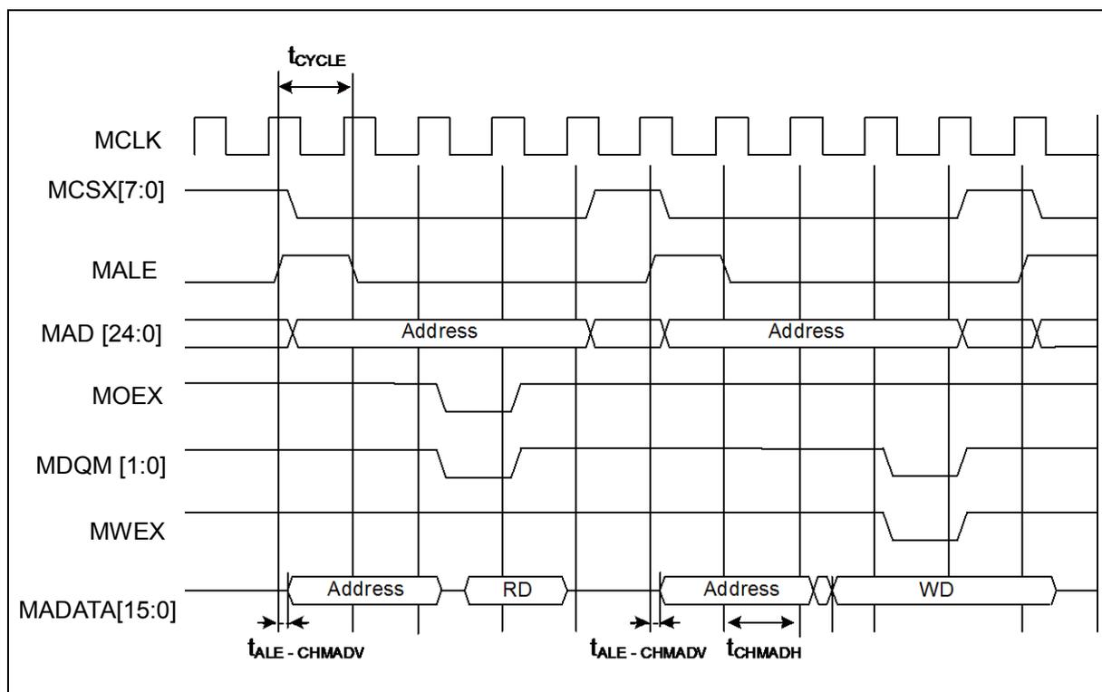
• Multiplexed Bus Access Synchronous SRAM Mode
