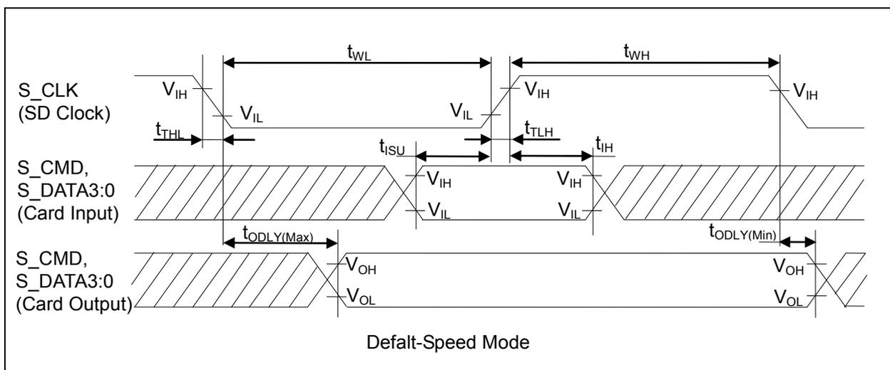
Note: The Card Input corresponds to the Host Output and the Card Output corresponds to the Host Input because this model is the Host.
