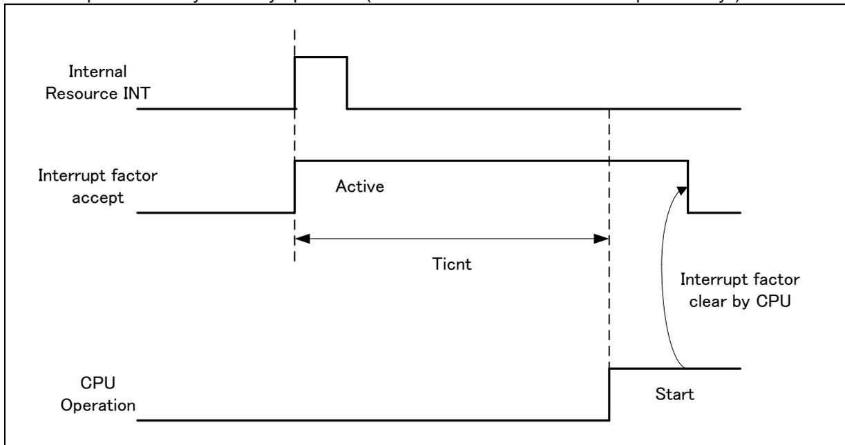
\*: Depending on the standby mode, interrupt from the internal resource is not included in the recovery cause.
