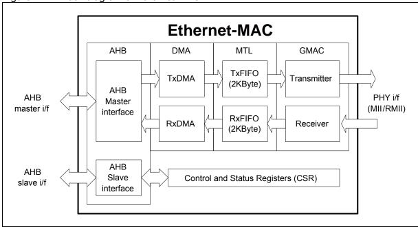
Figure 2-1 shows the block diagram of Ethernet-MAC. This section explains each function block.
