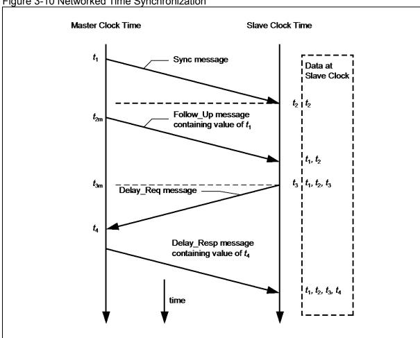
Figure 3-10 Networked Time Synchronization
