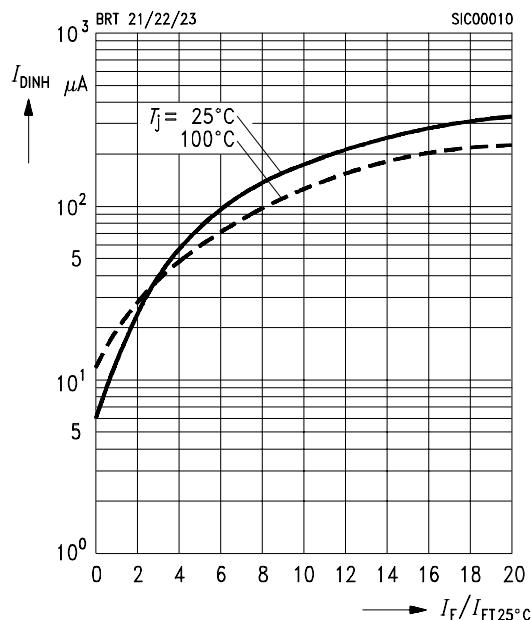
**Typ.static inhibit voltage limit** 5)
