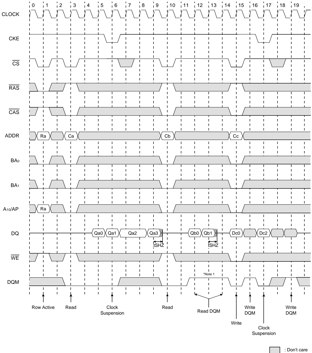
Clock Suspension & DQM Operation Cycle @CAS Latency=2, Burst Length=4
