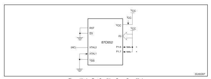
Figure 12.  $I_{CC}$  Test Condition, Power Down Mode All other pins are disconnected  $V_{CC} = 2V$  to 5.5V
