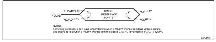
Figure 8. Float Waveform
