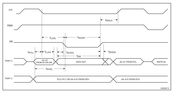
Figure 3. External Data Memory Write Cycle
