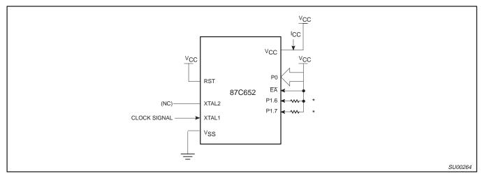
Figure 9. I<sub>CC</sub> Test Condition, Active Mode All other pins are disconnected
