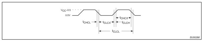
Figure 11. Clock Signal Waveform for  $I_{CC}$  Tests in Active and Idle Modes  $t_{CLCL} = t_{CHCL} = 10 ns$
