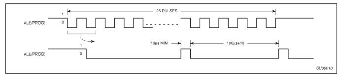
Figure 14. PROG Waveform
