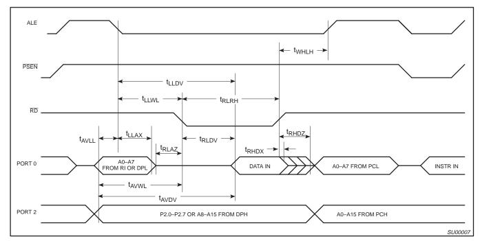
Figure 2. External Data Memory Read Cycle
