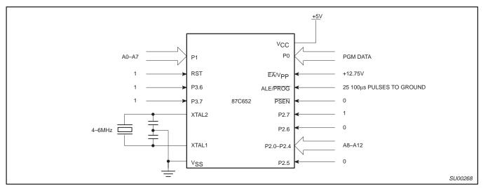
Figure 13. Programming Configuration
