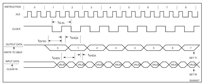
Figure 4. Shift Register Mode Timing
