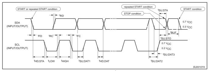
Figure 6. Timing SIO1 (I<sup>2</sup>C) Interface
