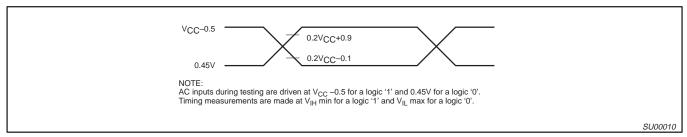
Figure 7. AC Testing Input/Output
