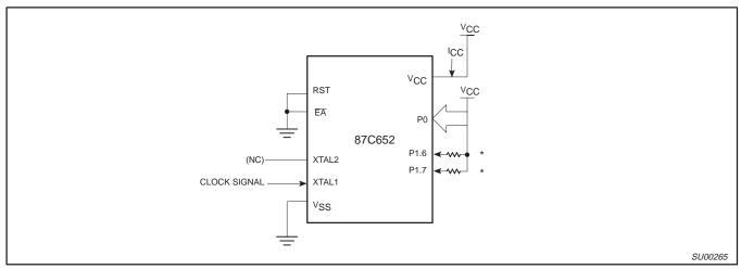
Figure 10. I<sub>CC</sub> Test Condition, Idle Mode All other pins are disconnected
