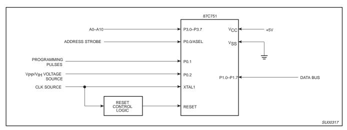
Figure 5. Programming Configuration
