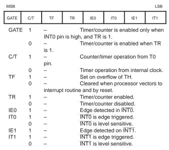
These flags are functionally identical to the corresponding 80C51 flags, except that there is only one timer on the 83C751 and the flags are therefore combined into one register.
