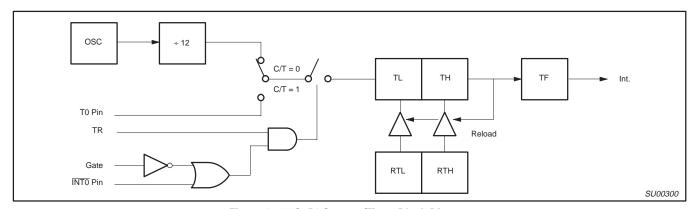
Figure 4. 83C751 Counter/Timer Block Diagram
