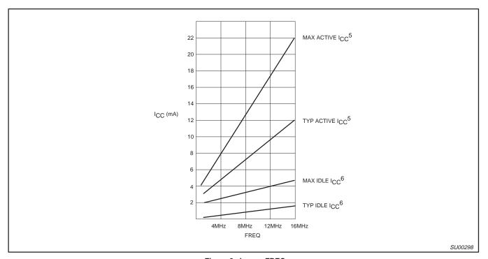
$\label{eq:local_local} Figure 2. \ I_{CC} \ vs. \ FREQ$   $\mbox{Maximum $I_{CC}$ values taken at $V_{CC}$ max and worst case temperature.}$   $\mbox{Typical $I_{CC}$ values taken at $V_{CC} = 5.0$V and $25^{\circ}$C.}$   $\mbox{Notes 5 and 6 refer to DC Electrical Characteristics.}$
