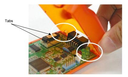
(5) Close the cover and tighten the screw.
