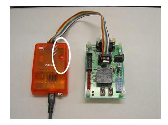
When turning on the power to the target system, POWER LED is ON (the QB-78K0MINI's power is ON and the target system's power is ON).
