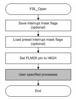
Figure 5-1 Flow of Self Programming Open Function
