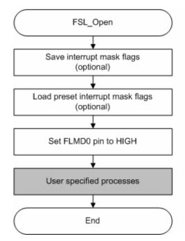
Figure 6-1 Flow of Self Programming Open Function
