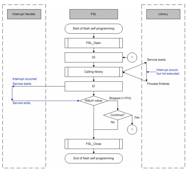
Figure 3-2 Flow of Processing in Case of Interrupt
