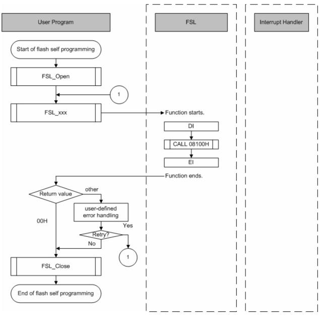
Figure 3-1 Flow of Processing without Interrupt
