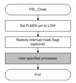
Figure 6-2 Flow of Self Programming End Function
