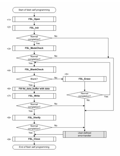
Figure 1-3 Flow of Self Programming (rewriting contents of flash memory)
