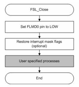
Figure 5-2 Flow of Self Programming End Function
