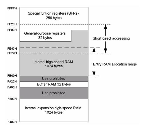
Figure 2-2 Allocation Range of Entry RAM
