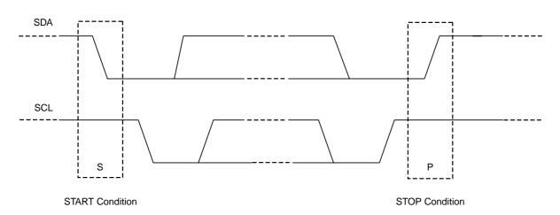
Figure 3-1: I<sup>2</sup>C START and STOP Conditions
