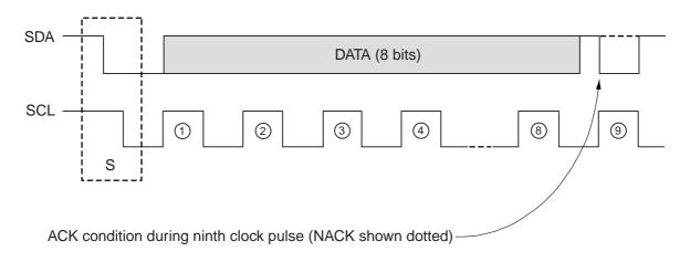
Figure 3-2: I<sup>2</sup>C ACK and NACK Conditions
