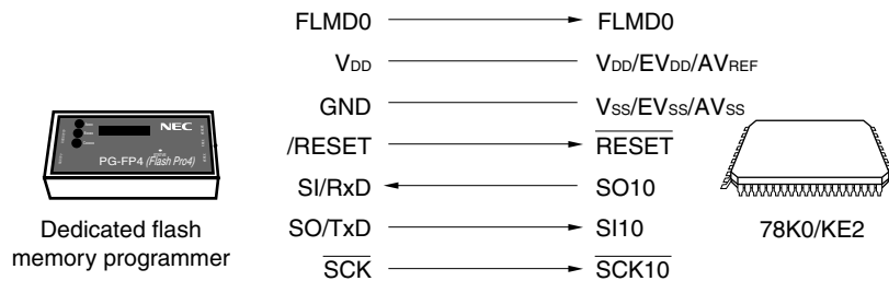
Figure 26-6. Communication with Dedicated Flash Memory Programmer (CSI10)
