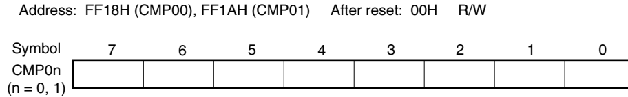
Figure 9-3. Format of 8-Bit Timer H Compare Register 0n (CMP0n)
