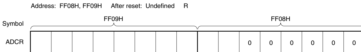
Figure 10-6. Format of A/D Conversion Result Register (ADCR)
