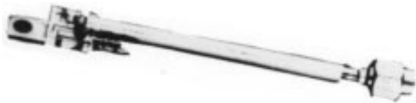
Figure 18. Photograph of CS-12 Impedance Measurement Probe
