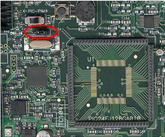
3. Be careful while inserting the PIC24FJ256GB110 PIM or any other appropriate PIM into Exp 16 board. Insure that no pins are bent or damaged during the process. Also insure that the PIM is not shifted in any direction and that all of the headers are properly aligned.
