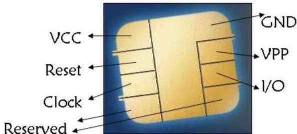
I/O: Input or Output for serial data to the integrated circuit inside the card.
