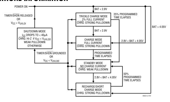
Figure 1. State Diagram for a Typical Charge Cycle
