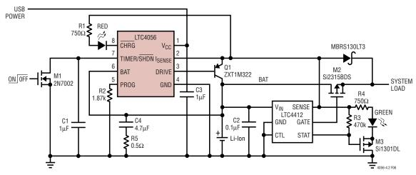
Figure 6. USB Charging and Automatic PowerPath Control with LTC4412 in Comparator Mode
