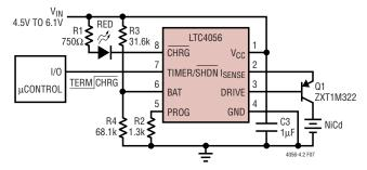
Figure 7. Nickel Chemistry Battery Charging
