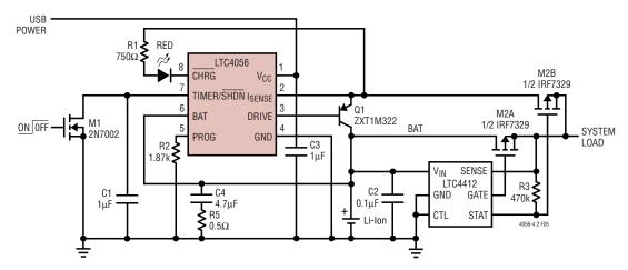
Figure 5. USB Charging and Automatic PowerPath Control with Auxiliary P-Channel MOSFET for Lowest Loss
