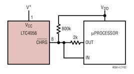
Figure 2. Using a Microprocessor to Determine CHRG State
