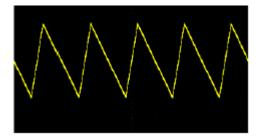
SOURce1:FUNCtion RAMP SOURce1:FUNCtion:RAMP:SYMMetry 25 SOURce1:FREQuency 1000
