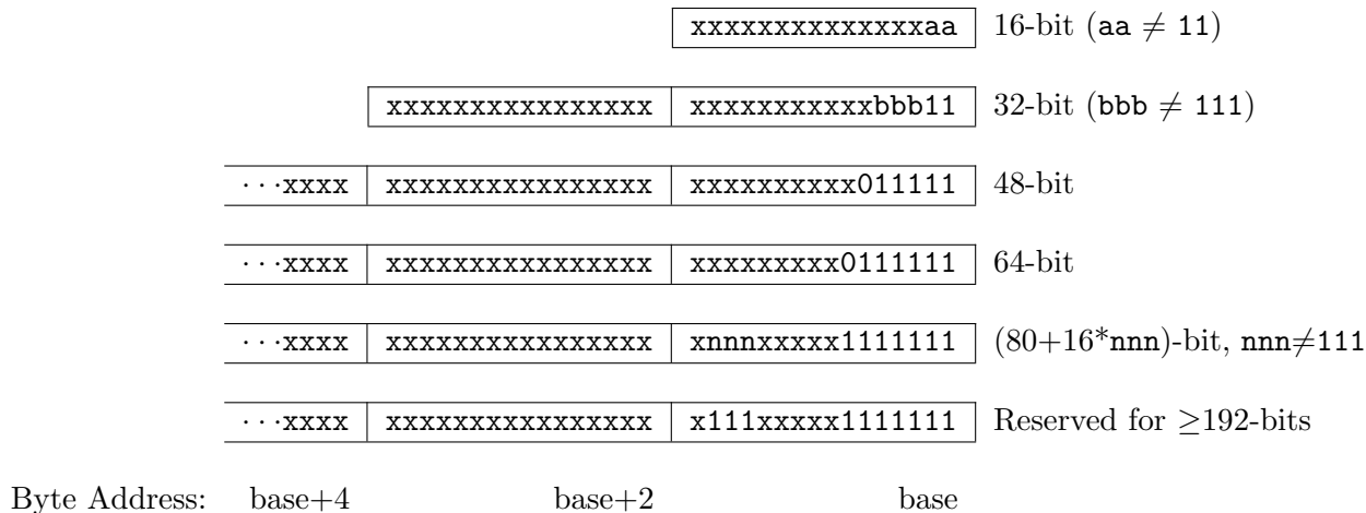
Figure 1.1: RISC-V instruction length encoding. Only the 16-bit and 32-bit encodings are considered frozen at this time.
