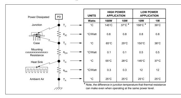
Calculations begin at the bottom of the chart and assume 25°C ambient temperature in these examples. Each component of thermal resistance produces a temperature rise equal to the product of power dissipated and thermal resistance. The temperature of the junction is equal to the product of power dissipated and the total thermal resistance (PD  $\cdot \theta_{1,v}$ ).
