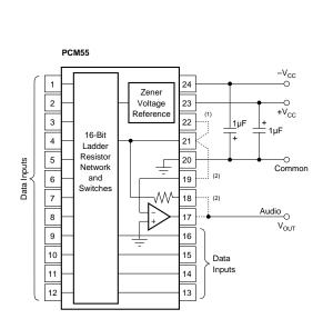
NOTES: (1) Connect for bipolar operation. (+V<sub>CC</sub>  $\geq$  8.5V for unipolar operation). (2) Connect for V<sub>OUT</sub> operation. When V<sub>OUT</sub> amp is not being used (I<sub>OUT</sub> mode), terminate with an external 3k $\Omega$  feedback resistor between pin 17 and pin 19, and a 1k $\Omega$  resistor between pin 19 and pin 20 to reduce possible noise effects.
