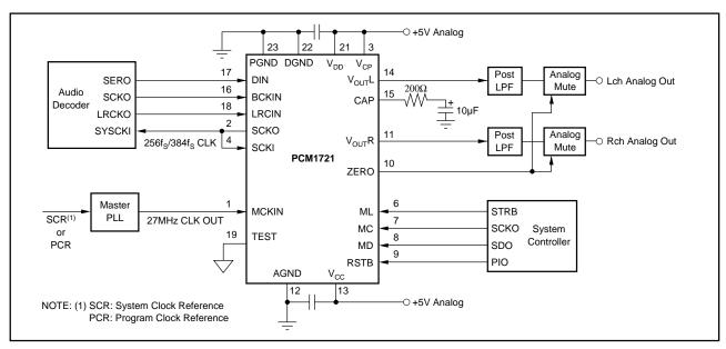
FIGURE 1. External Master Clock Input.
