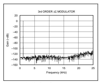
FIGURE 16. Quantization Noise Spectrum.
