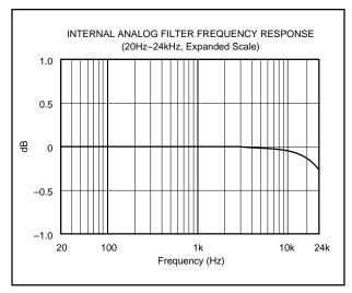
FIGURE 9. Low Pass Filter Frequency Response.
