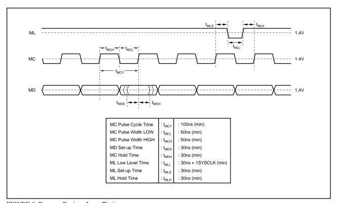
FIGURE 8. Program Register Input Timing.
