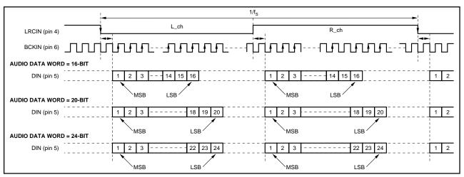
FIGURE 5. "I2S" Data Input Timing.
