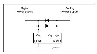
FIGURE 14. Latch-up Prevention Circuit.
