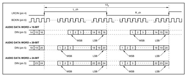
FIGURE 4. "Normal" Data Input Timing.
