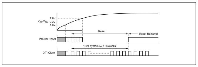
FIGURE 12. Internal Power-On Reset Timing.
