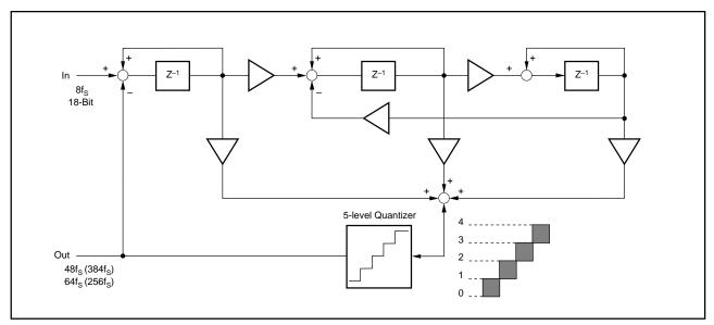
FIGURE 15. 5-Level  $\Delta\Sigma$  Modulator Block Diagram.
