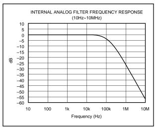
FIGURE 10. Low Pass Filter Wideband Frequency Response.
