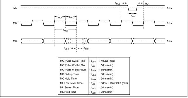
FIGURE 6. Serial Interface Timing.
