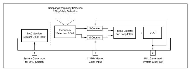
FIGURE 2. PPL Block Diagram.
