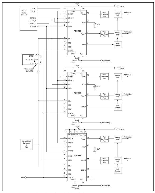
FIGURE 17. Connection Diagram for a 6-Channel AC-3 Application.
