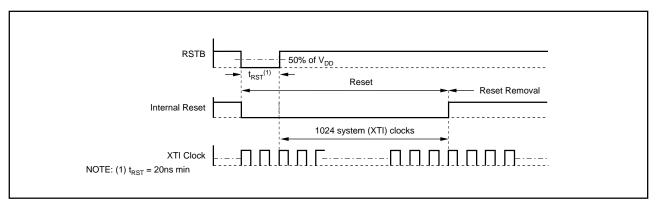
FIGURE 13. RSTB-Pin Reset Timing.
