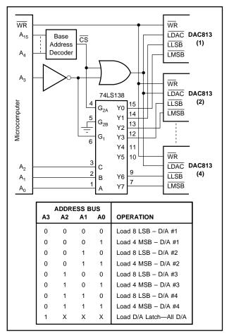
FIGURE 9. Interfacing Multiple DAC813s to an 8-Bit Bus.
