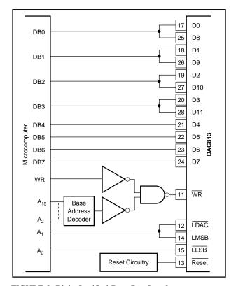
FIGURE 8. Right-Justified Data Bus Interface.
