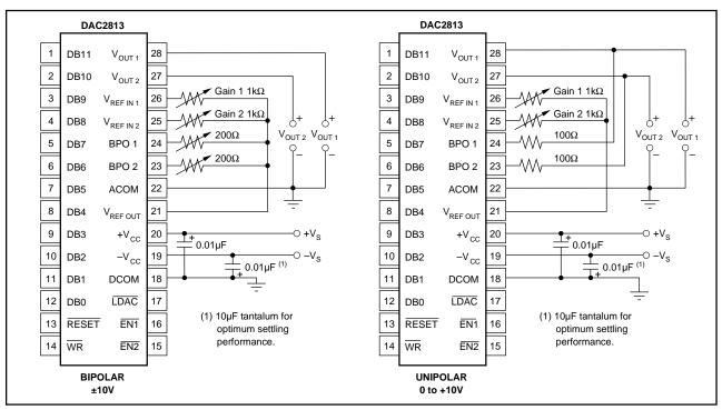
FIGURE 3. DAC2813 Power Supply, Output Range, Gain and Offset Adjust Connections. Unipolar output connected DAC2813s have Gain Adjust only.
