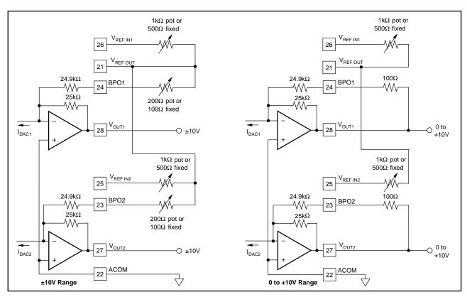
FIGURE 4. DAC2813 Output Amplifier Range Connnections.
