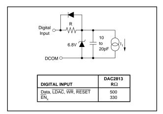
FIGURE 1. Equivalent Digital Input Circuit.
