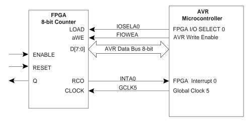
The block diagram shows the connections used in this example, all interface connections are implemented using dedicated resources. This example makes use of the AVR-FPGA Data Bus, one FPGA Interrupt and one I/O Select signal.
