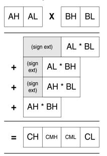
**16-bit x 16-bit = 16-bit Operation**This operation is valid for both unsigned and signed numbers, even though only the unsigned multiply instruction (MUL) is needed. This is illustrated in Figure 3. A mathematical explanation is given:
