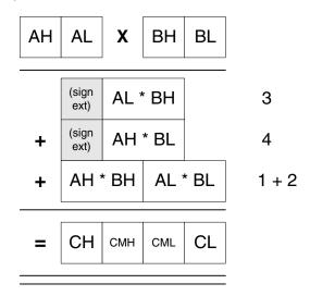
The 32-bit result of the unsigned multiplication of 672 and 1844 will now be in the registers R19:R18:R17:R16. If "muls16x16\_32" is called instead of "mul16x16\_32", a signed multiplication will be executed. If "mul16x16\_16" is called, the result will only be 16 bits long and will be stored in the register pair R17:R16. In this example, the 16-bit result will not be correct.
