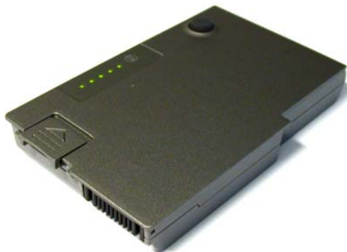
Figure 1-1. Smart battery from the author's laptop
