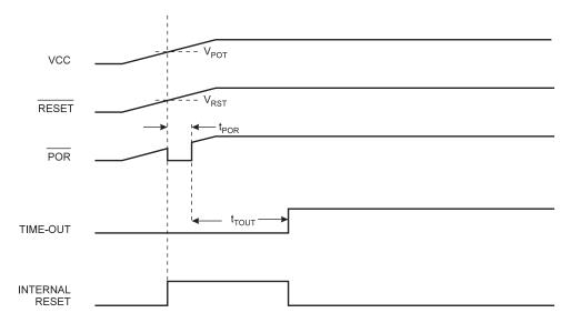
Figure 28. MCU Start-Up,  $\overline{\text{RESET}}$  Tied to  $V_{CC}$  or Unconnected. Slowly Rising  $V_{CC}$
