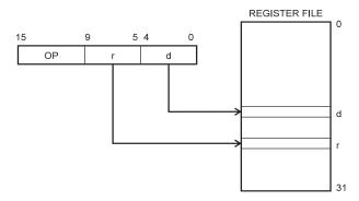
Figure 10. Direct Register Addressing, Two Registers
