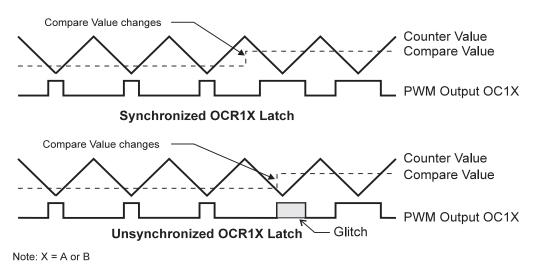
Figure 37. Effects on Unsynchronized OCR1 Latching
