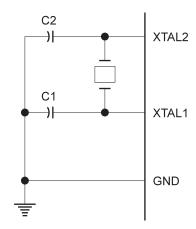
Figure 2. Oscillator Connections
