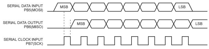
Figure 65. Serial Downloading Waveforms
