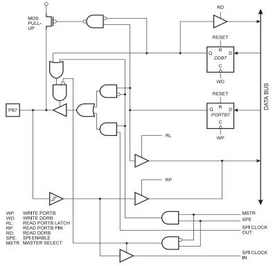
Figure 53. PORTB Schematic Diagram (Pin PB7)
