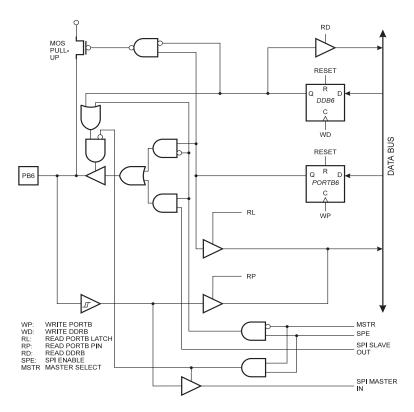
Figure 52. PORTB Schematic Diagram (Pin PB6)
