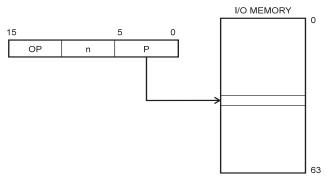
Figure 11. I/O Direct Addressing
