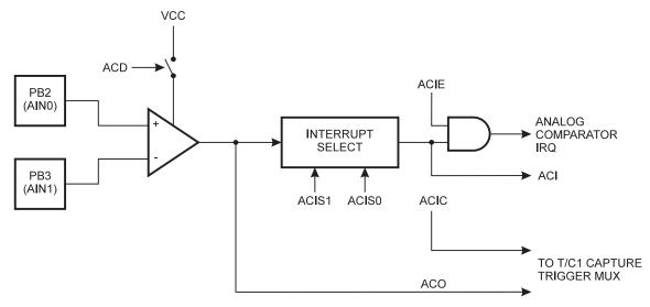
Figure 46. Analog Comparator Block Diagram
