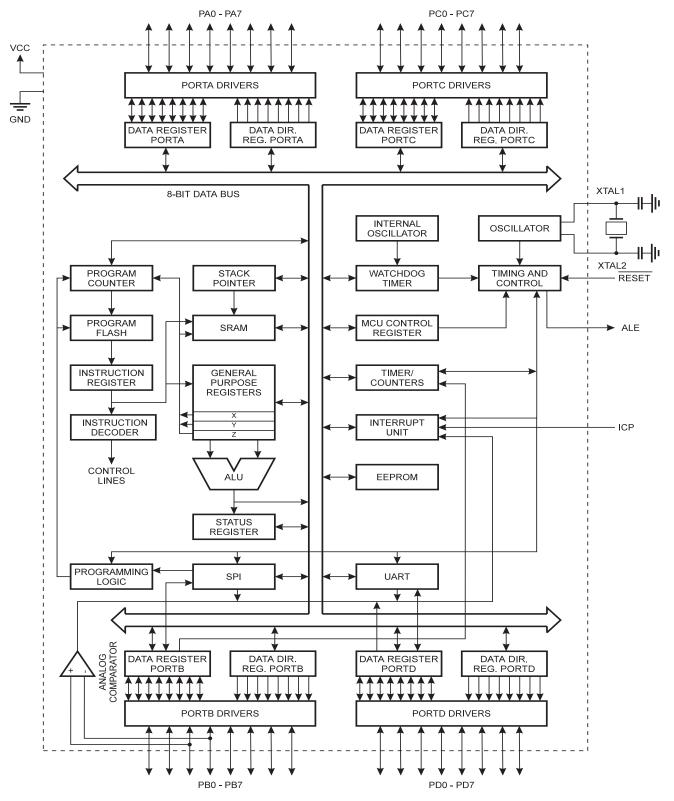
Figure 1. The AT90S4414 Block Diagram
