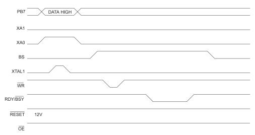
Figure 64. Programming Flash High Byte
