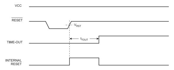
Figure 30. External Reset During Operation
