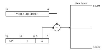
Figure 13. Data Indirect with Displacement
