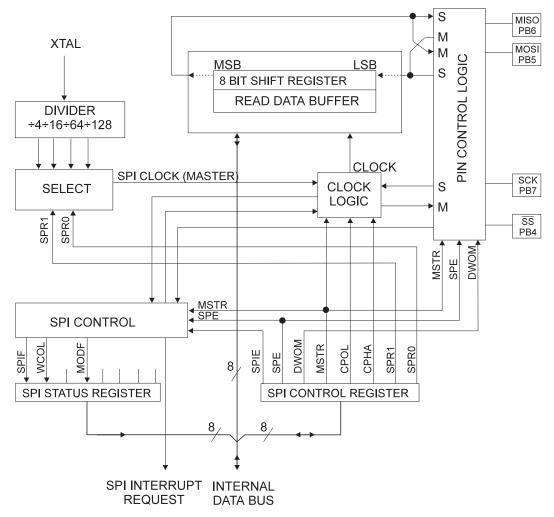
Figure 39. SPI Block Diagram
