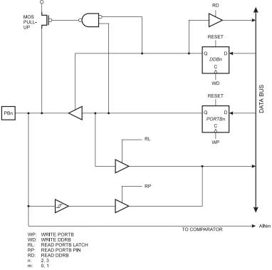
Figure 49. PORTB Schematic Diagram (Pins PB2 and PB3)
