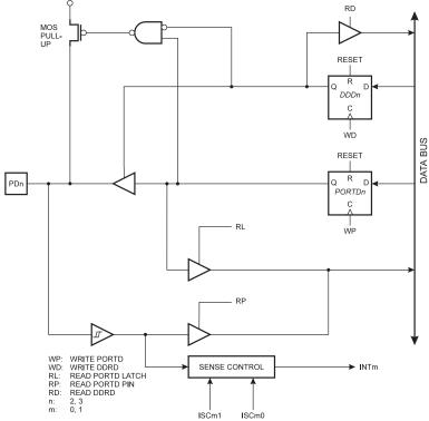
Figure 57. PORTD Schematic Diagram (Pins PD2 and PD3)
