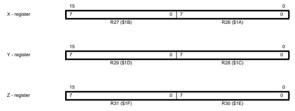
Figure 7. The X, Y and Z Registers
