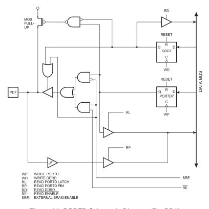
Figure 61. PORTD Schematic Diagram (Pin PD7)
