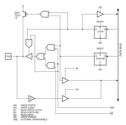
Figure 60. PORTD Schematic Diagram (Pin PD6)
