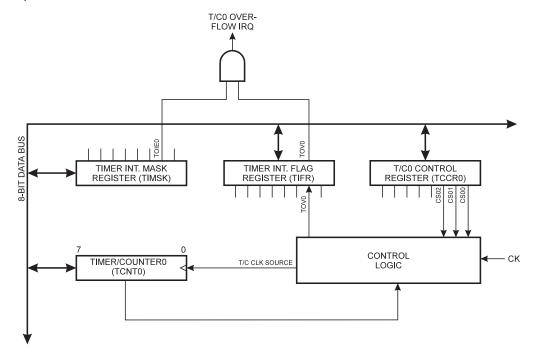
Figure 33. Timer/Counter0 Block Diagram
