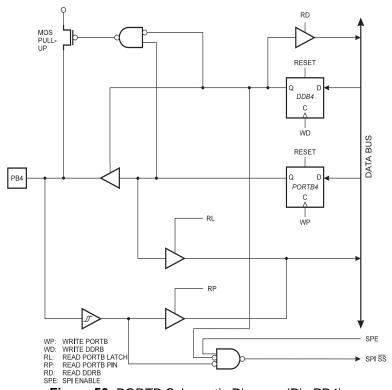
Figure 50. PORTB Schematic Diagram (Pin PB4)
