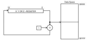
Figure 16. Data Indirect Addressing With Post-Increment
