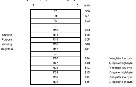
Figure 6. AVR CPU General Purpose Working Registers
