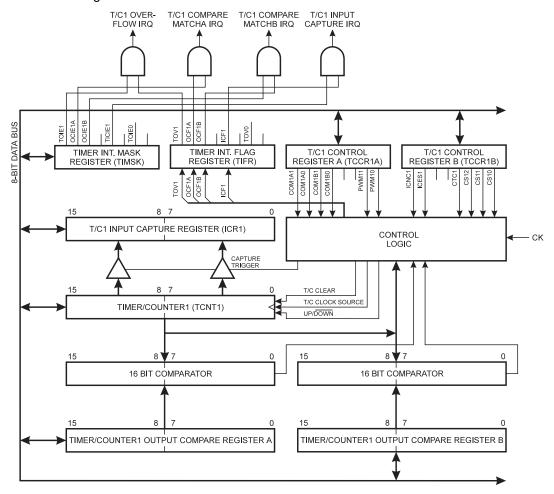
Figure 34. Timer/Counter1 Block Diagram
