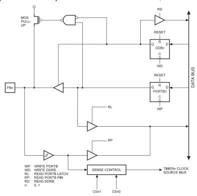
Figure 48. PORTB Schematic Diagram (Pins PB0 and PB1)
