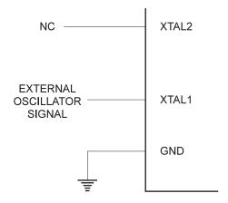
Figure 3. External Clock Drive Configuration
