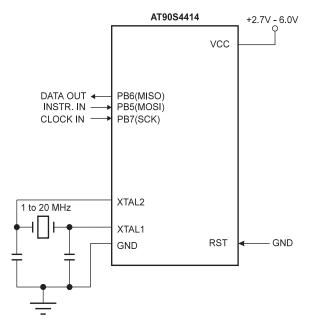
Figure 66. Serial Programming and Verify
