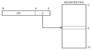
Figure 9. Direct Single Register Addressing
