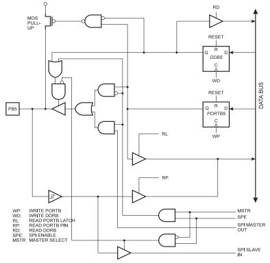
Figure 51. PORTB Schematic Diagram (Pin PB5)
