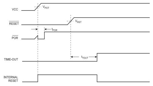
Figure 29. MCU Start-Up, RESET Controlled Externally
