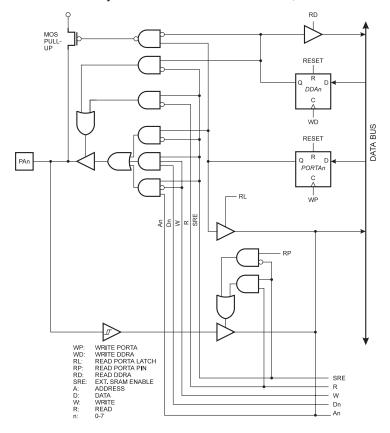
Figure 47. PORTA Schematic Diagrams (Pins PA0 - PA7)
