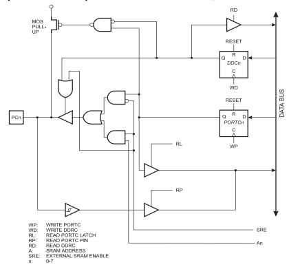
Figure 54. PORTC Schematic Diagram (Pins PC0 - PC7)
